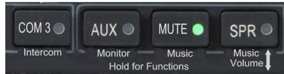
tercom audio distribution, and allows the crew to mute passengers' intercom feed when radios are active.
