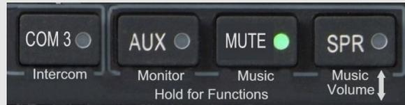
“**Monitor**” activates a **Monitor Mode**. In this case, the audio from the COM radio that is selected for transmit will mute the other COM audio when it is active. For example, if COM 1 is selected to transmit to ATC, but COM 2 is receiving weather information; the ATC will mute the audio from the weather while ATC is transmitting. In Monitor mode, the RCV COM indicator will blink every few seconds as a status indication. Monitor mode is set to off when the unit is turned off.
