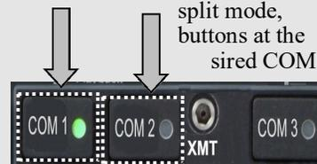
1 or COM 2 XMT button. When you activate the Split mode, the intercom is inhibited to avoid confusion with multiple conversations. To reactivate the intercom, press the Mute button. Note: Split Mode does not turn off Nav, ADF, or Aux selected audio to pilot. However, the copilot will only hear the selected com receiver and unswitched inputs.
