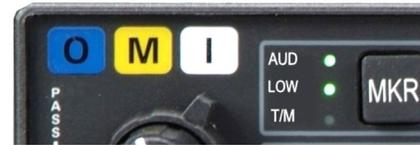
The **MKR** button is also used to test the indicator lamps and mute the marker audio. Pressing the **MKR** button for one second will cause the marker audio to mute. The next beacon received will re-activate the audio.
